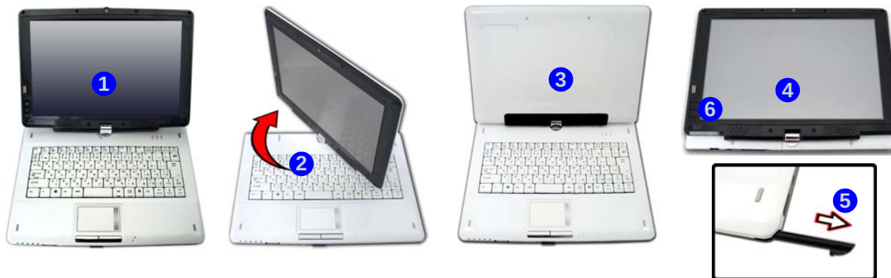
Figure 2 - Rotating the LCD Panel Into Tablet Mode
