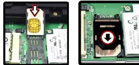
Figure 18 USIM Card Insertion & SIMLOCK Lock
