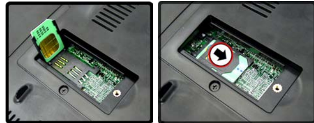
Figure 13 - Insert the USIM Card & Lock the SIM-LOCK
