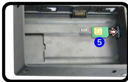
Figure 1 - 18 USIM Card & Battery Insertion
